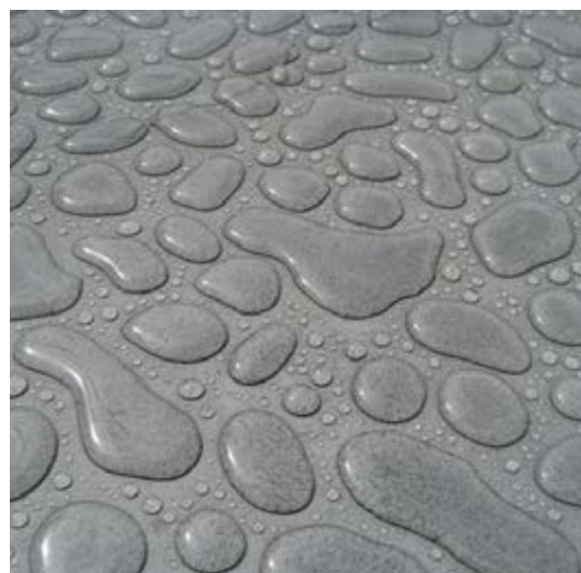
Hydrophobized concrete surface
